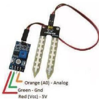
Fig 5: Soil Moisture Sensor
