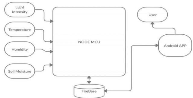
Fig. 2: Technical Block Diagram
